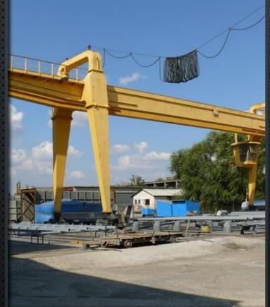
Own outdoor and indoor warehouse with gantry cranes for loading and discharging activity is connected to the national railway network and is able to accept and store metals and steel structures, pipes and pipe fittings, cables, cable drums, and auxiliary and ancillary materials for performing the Company's activities and for materials for its partners
